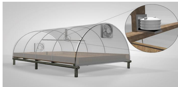
Fig. 9. Final design model with sensor shield detail.
